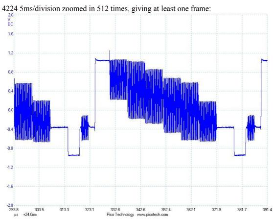
As you can see the 2203 is good only for shorter time bases, whilst the 4224 gives very good detail out of the longer time bases. The 3224 and 3206 give also good detail on the longer time bases, however not as good as the 4224. You may have also noticed that the 3224 and 4224 give more detail on the voltage.
