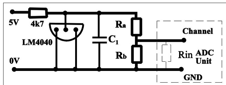
The 5V supply can be taken from the terminal block. It is converted to a stable and precise 2.5V using the LM4040 voltage reference device (Maplin part number ARC81).
