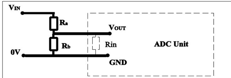
There are positions on the terminal board for resistors Ra and Rb. **\*NOTE\*** There is a thin track on the terminal board under position Ra which must be cut with a sharp knife before the potential divider will work.
