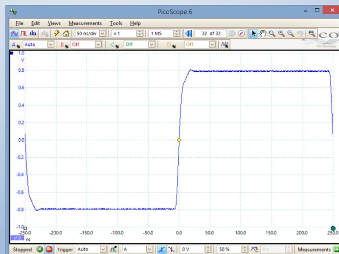
The above example shows that, even with PicoScope's optimized 20 Hz display update rate, only a tiny proportion of the input signal ever appears on the display. Even if the glitch does appear, you might not see it after waiting for 14 hours.
