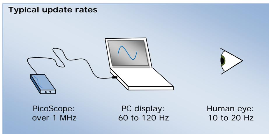
The data acquisition hardware can often capture millions of waveforms per second. Clearly, the digital oscilloscope needs to reduce the amount of captured data before displaying it, but how can it do this without throwing away important information? The answer is: it's up to you, the user. If you understand how to use the scope to filter out unwanted data, you will be able to maximize your chances of finding intermittent events such as glitches.
