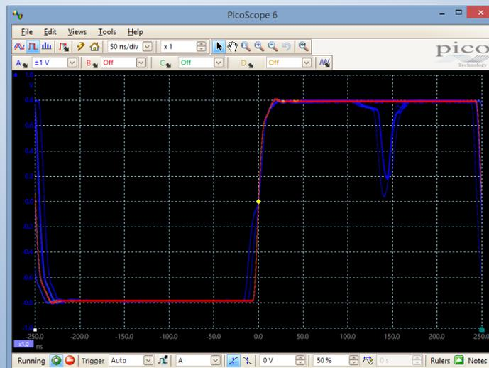
The hottest colors (such as red) indicate the densest areas of data where the majority of the waveforms are located. The coolest colors (such as blue) indicate transient events such as glitches and jitter.
