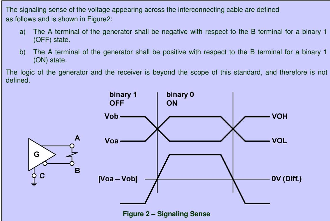
Texas Instruments datasheets for RS-485 transceivers follow the convention that A is the non-inverting pin and B is the inverting pin.
