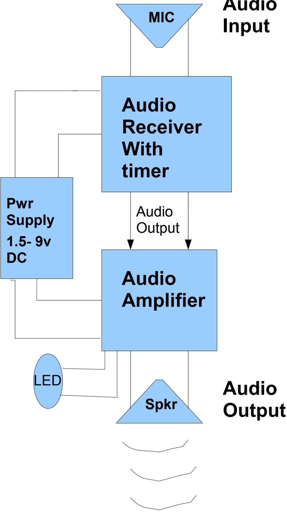
Receiver: Listens for repetitive audio Clicks. (like metronome) After a variable time period of 5-10 seconds if the clicks don't go away, the receiver will begin to output the audio clicks to an audio amplifier. The audio amplifier will begin to output the clicks at a much higher db level (+ 20db.) An LED will blink on and off in sync with the audio clicks. Every 5 seconds, the receiver will cease output and revert to listen mode.
