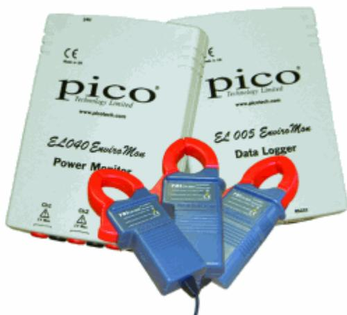
The current monitoring kit provides a complete solution to measuring three channels of mains current. This could typically be applied to measuring and balancing three-phase supplies or monitoring the increase / decrease in current drawn from mechanical equipment to aid maintenance schedules.
