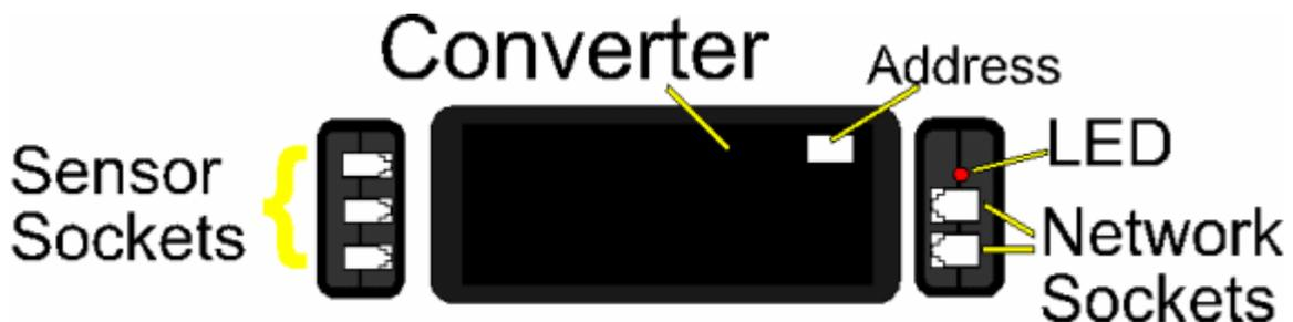
The LED flashes continuously immediately after the system is turned on. Once the system is running normally, the light goes out and, thereafter, flashes briefly each time the converter takes a reading.
