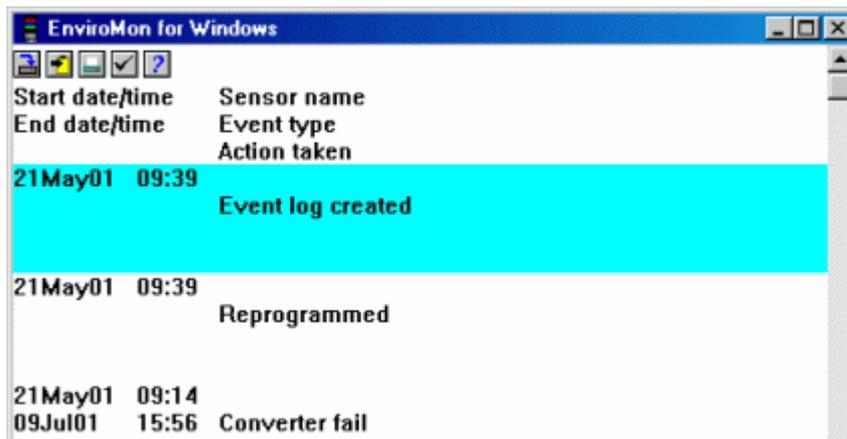
There are two or four lines of text for each event. At the left is the start and end date/time: the end date/time is omitted if the fault is still active. Next to these are the sensor name and a description of the fault. If **Show action taken** is enabled, the action taken will be displayed beneath the fault description.
