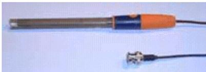
pH is measured using a standard electrode with a BNC connector. Pico supplies a robust epoxy-bodied pH electrode ideal for educational use. It covers the full 0 to 14 pH range.
