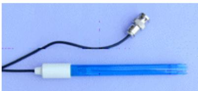
Pico supplies two different makes of pH electrode. Both operate in exactly the same way and are interchangeable in use. Before using your electrode please remove either the protective cap (top photograph) or storage bottle (bottom photograph).
