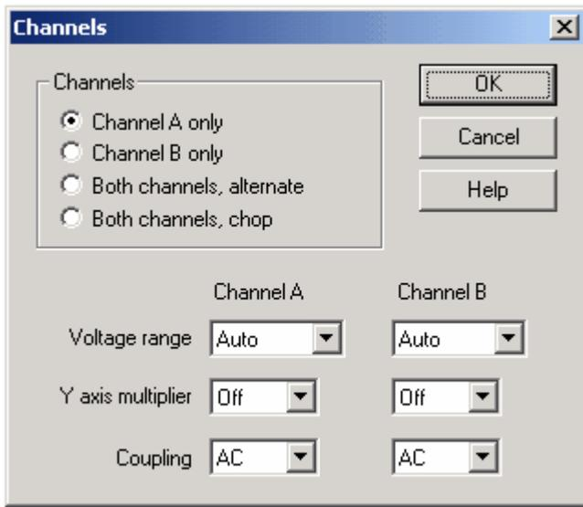
This dialog box enables you to select which input channels to display in the active window and to set the input voltage ranges.
