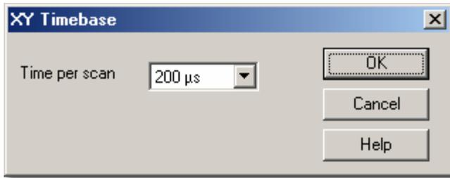
This dialog box controls the timebase for the active XY scope window.
