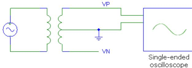
With a differential oscilloscope, you can directly measure the secondary voltage by connecting the positive probe to  $V_P$  and the negative to  $V_N$ . This is shown in the diagram below. A ground connection is not essential, although it is a good idea to use a shielded cable grounded at one end in order to prevent electromagnetic noise coupling into the cable.
