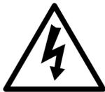
The accessories supplied with the PicoScope 3425 are rated for safe working at the maximum voltages stated in the [Specifications](#). For your safety, if you use your own accessories with this oscilloscope, you **must** ensure that they are rated for the voltage you are measuring.
