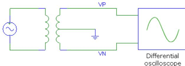
Differential oscilloscopes have many other applications where the voltage to be measured is not referenced to ground, or where it is not desirable to connect the scope ground to the ground of the device under test.
