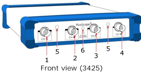
1. **Ch A.** Input channel A. As this is a [differential oscilloscope](#), the channels have non-standard input impedances and **cannot be used with passive attenuated scope probes** such as the x1/x10 probes supplied with conventional oscilloscopes.
