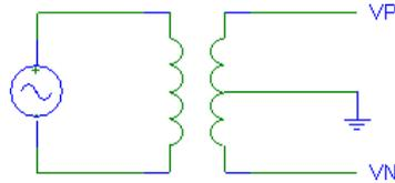
A single-ended oscilloscope can only measure a signal with reference to ground, so you need to connect the scope's ground clip to the centre of the secondary. You can then measure either  $V_P$  or  $V_N$  with respect to ground, but not the total voltage across the secondary. The diagram below shows a single-ended scope connected between  $V_P$  and ground:
