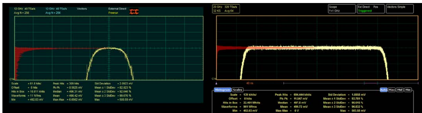
Figure 4 – Faster sampling and better sensitivity on PicoScope 9300 Left: PicoScope 9200 – 10 ps/div, 2 mV/div (200 fs and 40 \mu V resolution) Right: PicoScope 9300 – 5 ps/div, 1 mV/div (64 fs and 40 \mu V resolution)
