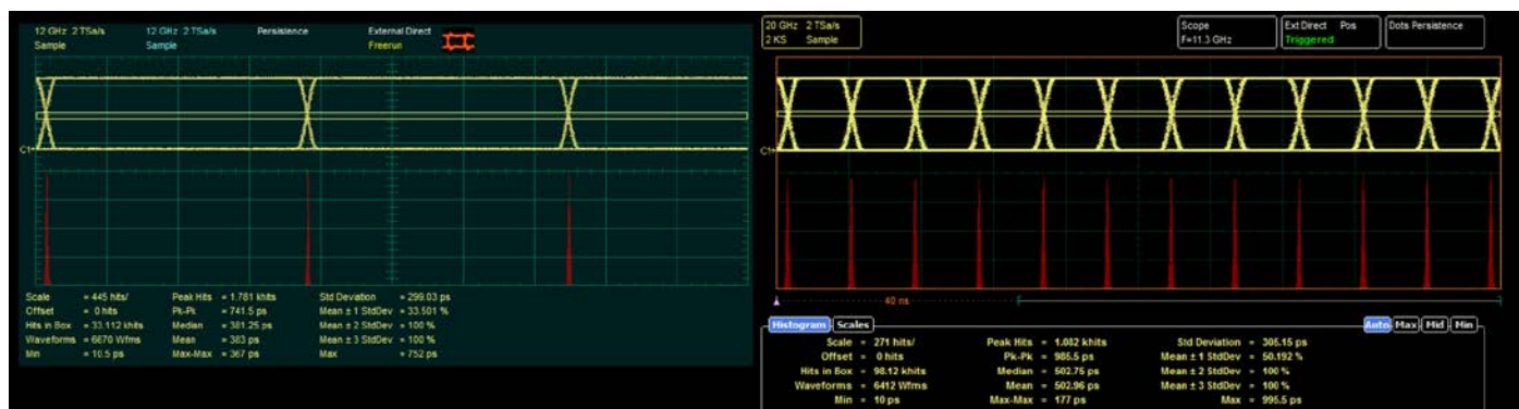
Figure 3 - Faster serial data clock recovery with the PicoScope 9300 Left: PicoScope 9200 Series. Right: PicoScope 9300 Series.
