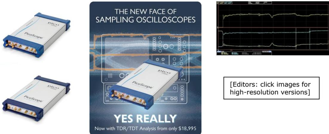
Newly released, the PicoScope® 9300 Series TDR/TDT Sampling Oscilloscopes can perform time-domain reflectometry and transmission mismatch and network analysis on high-frequency cables, PCBs, backplanes and interconnections. Their built-in differential fast edge generators have a rise time of 65 ps at up to 6 V (PicoScope 9311) or 40 ps at over 250 mV (PicoScope 9312 via plug-in pulse heads), providing a typical distance-to-fault resolution down to 10 mm.
