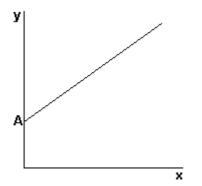
The above linear and non-linear responses could have a voltage, current, resistive or other type of offset that may need taking into account. It is quite usual to see offsets in output signals from sensors.
