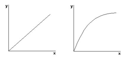
A linear response is one whose output-versus-input graph is a straight line. An example of this type of response is a photodiode.
