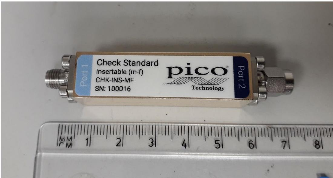
*Figure 2 – Pico Technology insertable (m-f) check standard*
