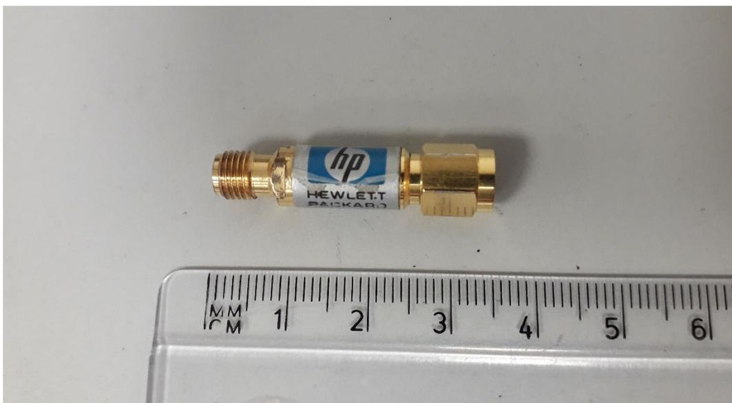
Figure 7 – Hewlett Packard 20 dB attenuator
