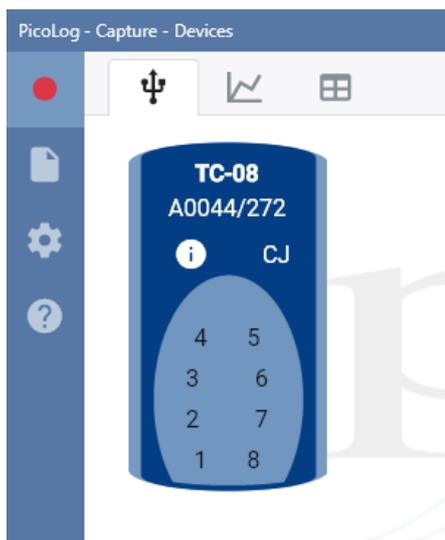
1. Select the channel corresponding to the location you chose for the thermocouple. The channel setup dialog will then display, allowing you to configure the channel. You can type in a channel **Label** and choose a channel **Color**, **Sample interval** and **Input type** (thermocouple type). You also have an advanced option to set **Custom scaling**:
