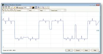
All units have a built-in function generator with at least sine, square, triangle and DC modes. As well as basic controls to set level, offset and frequency, more advanced controls allow you to sweep over a range of frequencies and trigger the generator from a specified event. Combined with the spectrum peak hold option, this becomes a powerful tool for testing amplifier and filter responses.
