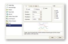
the data you need. All advanced trigger types have adjustable thresholds and hysteresis. The MSOs have a further set of *digital* triggers that can detect any data pattern with optional edge-sensitivity. The *logic* trigger applies the selected Boolean operation to any number of analog, EXT or MSO digital inputs.
