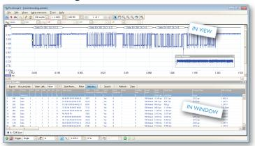
The PicoScope 3000 Series, with its deep memory, is ideal for serial decoding as it can capture thousands of frames of uninterrupted data. Protocols currently included are I<sup>2</sup>C, I<sup>2</sup>S, SPI, RS232/UART, CAN, LIN and FlexRay. Expect this list to grow with free software updates.
