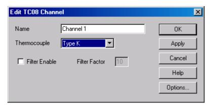
8. From the **Thermocouple** drop-down list, select the thermocouple type you wish to use, then click **OK.** The recorder view should now display the temperature.
