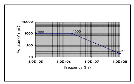
The derating curve for absolute maximum input voltage is as follows:
