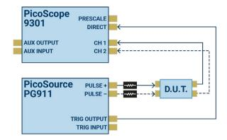
Single-ended and differential connections for TDT testing, using a PicoSource pulse generator with SRD outputs
