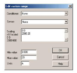
The custom range on the left scales the mV output from the current clamp on the 1 mV / 10 mA setting. PicoScope will show the output from the current clamp in the range 0 to 20 amps.
