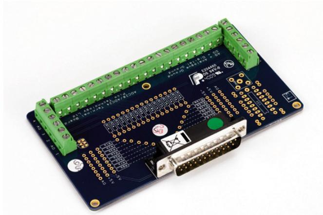
Additionally, the ADC-24 has four configurable digital input/output channels that can be used to control alarms or other devices. The flexibility of the ADC-20 and ADC-24 allows you to use these precision data loggers as an advanced multichannel data acquisition system with a low cost per channel.
